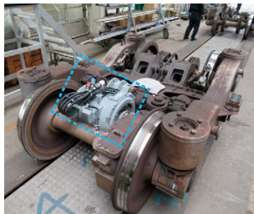
Installation of SynRM on a trial basis
