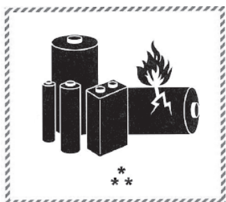
Figure 1: Lithium battery mark example
