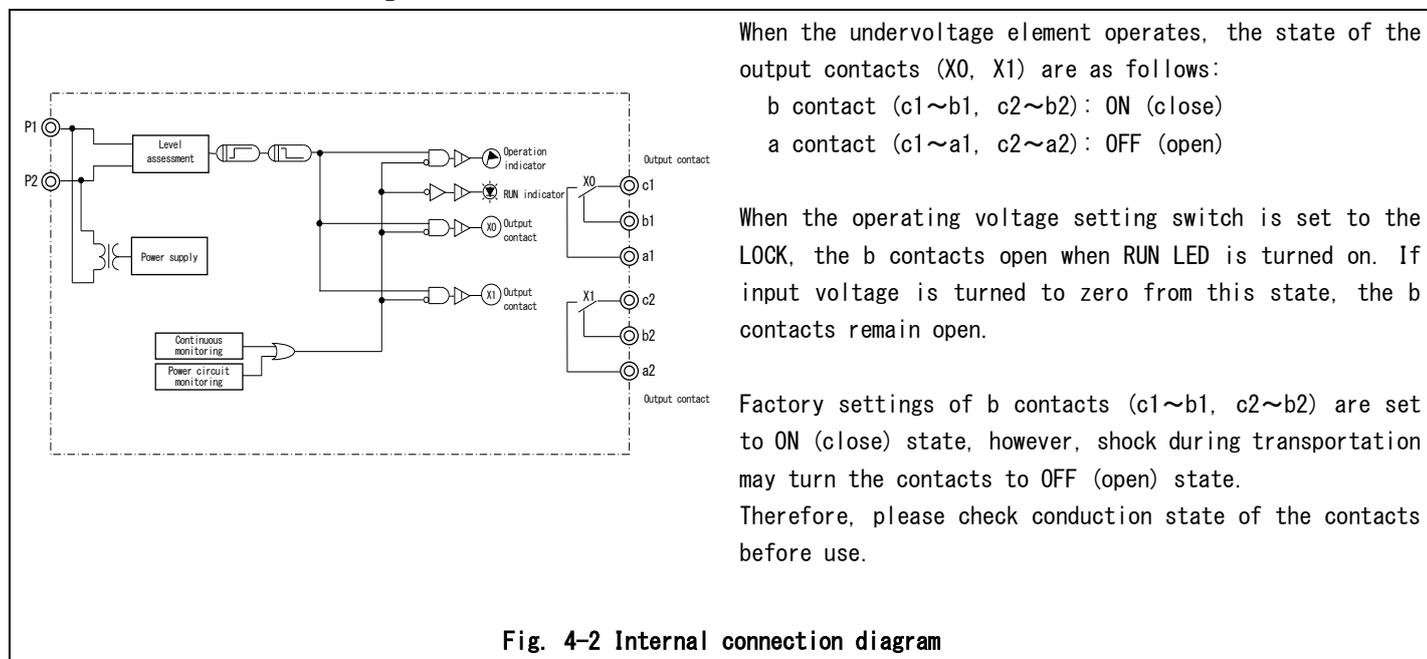
When the undervoltage element operates, the state of the output contacts (X0, X1) are as follows:
