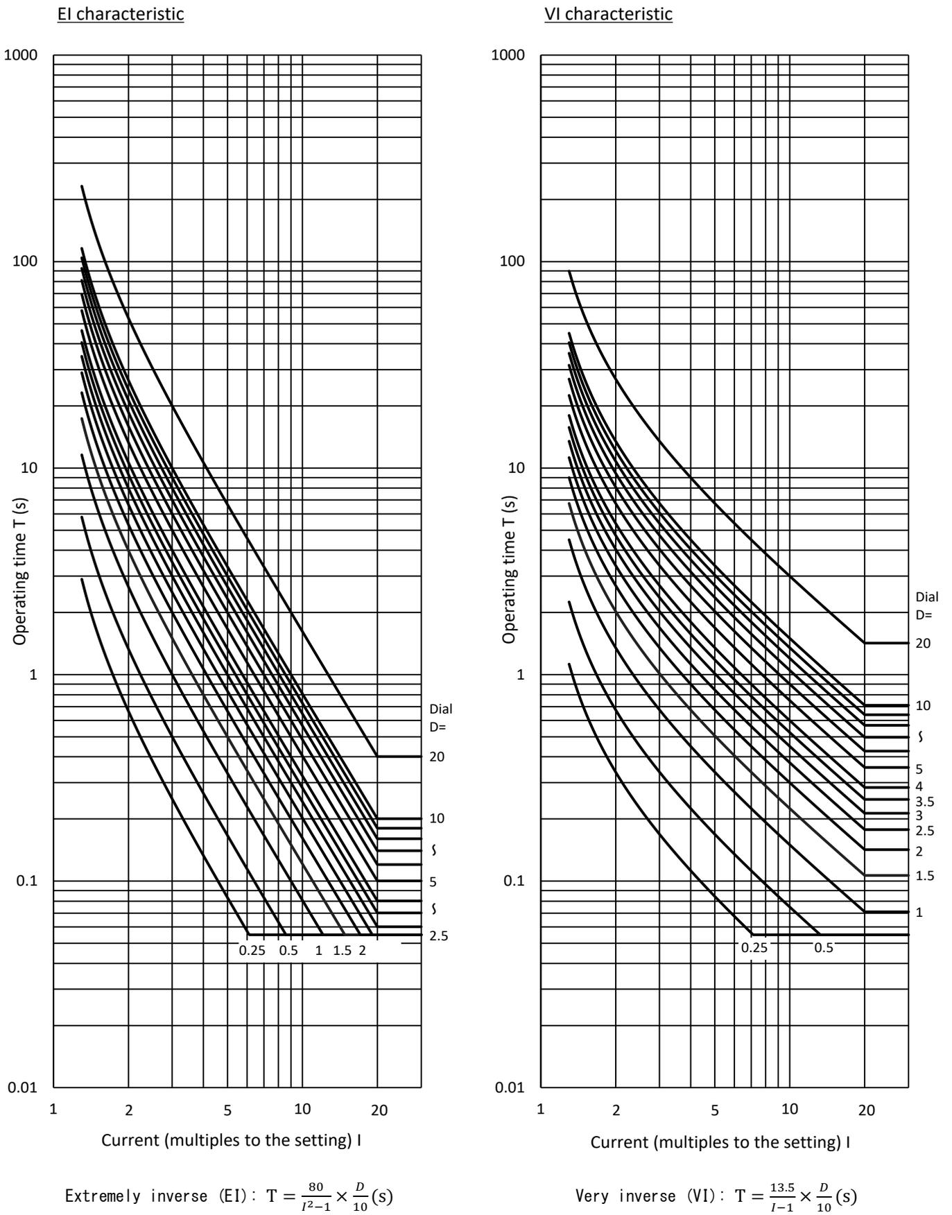
Fig. 1-1-1 Operating time characteristics
