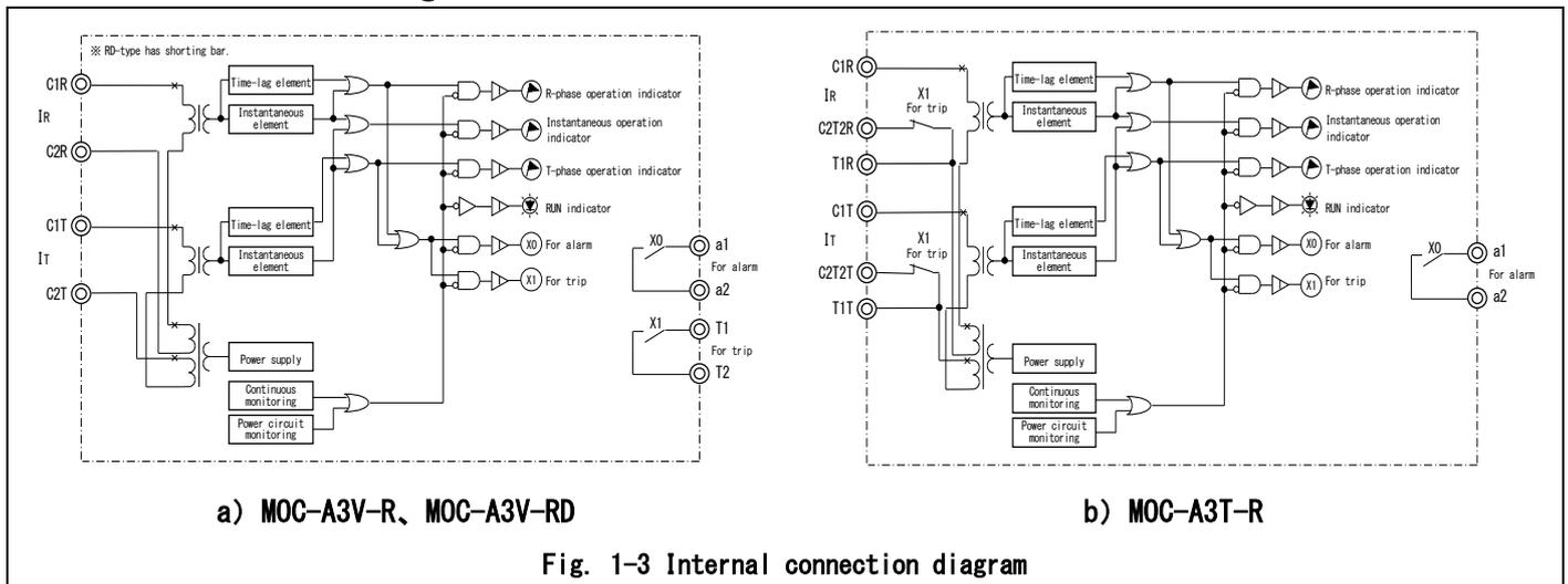
Fig. 1-3 Internal connection diagram
