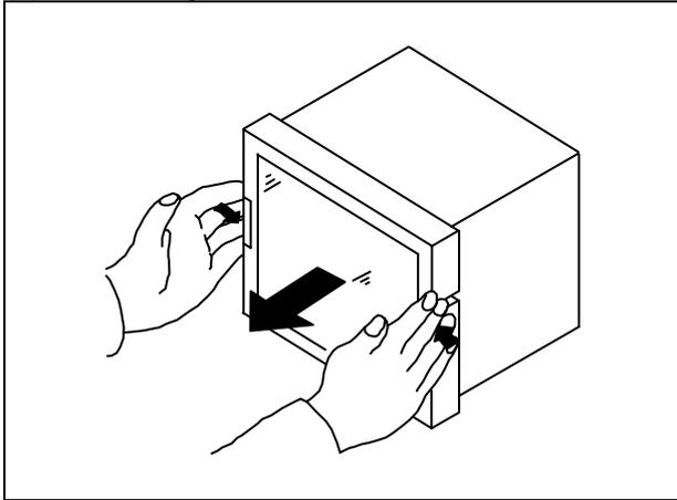
Hold the **lock levers**, which are located at both sides of the cover, on their front sections. Take off the cover **straight toward you** while pushing the levers **inwards**.
