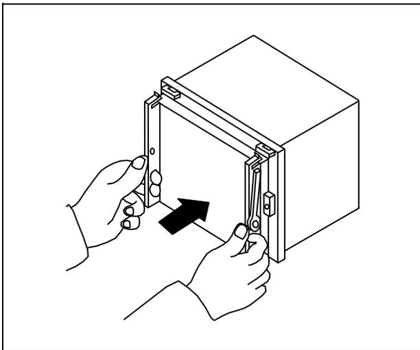
**Under holding the auxiliary levers locked status** by the with-holder (not to let the draw-out auxiliary levers fall down), **Insert the sub unit into the case until the auxiliary levers touch the metallic parts** while pressing the handles located on both sides of the front of the sub unit.
