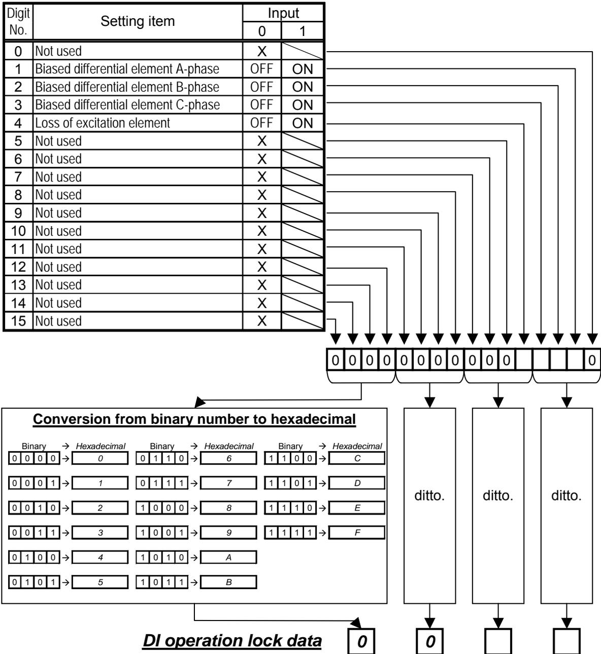
When the product is shipped from the factory, DI1 is set to lock of bias differential element lock, and DI2 is set to lock of loss of excitation like the following table.
