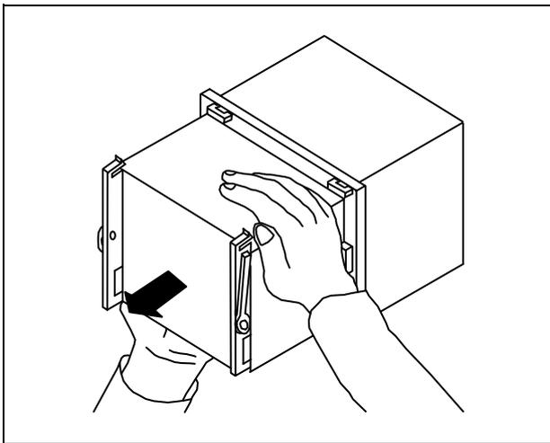
When about a half portion of the sub unit is pulled out of the case, just stop the drawing motion. Then, **hold the top and bottom of the sub unit to pull it out completely**, in order to prevent the unit from falling.
