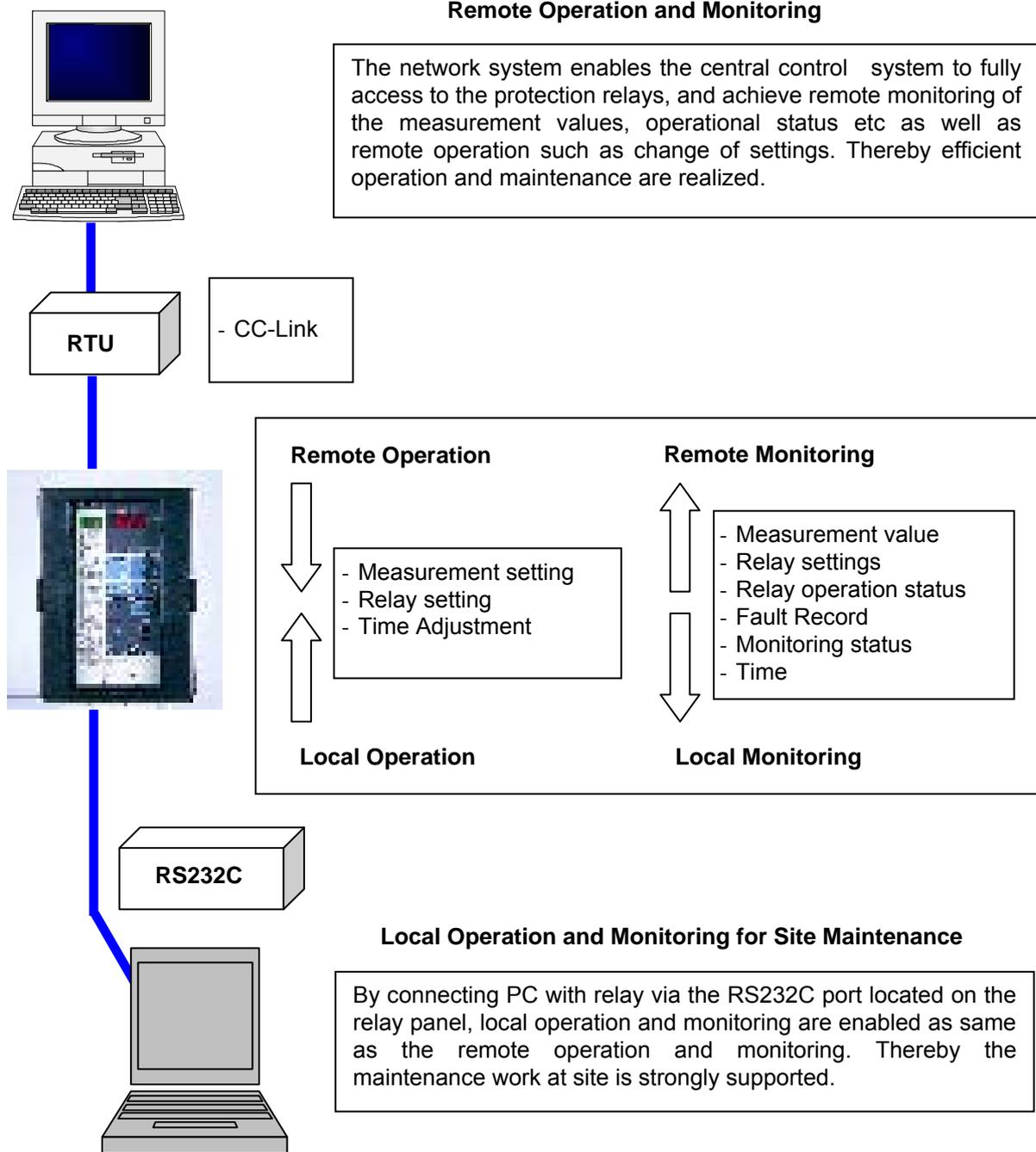
**Figure 4-16 Example of communication network system configuration**
