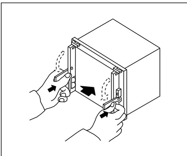
**More fully insert the sub unit into the case until the auxiliary levers fall down automatically and catch the metal holes inside with its hooks.** (**Rotating angle is from 180° to approx. 45°**)
