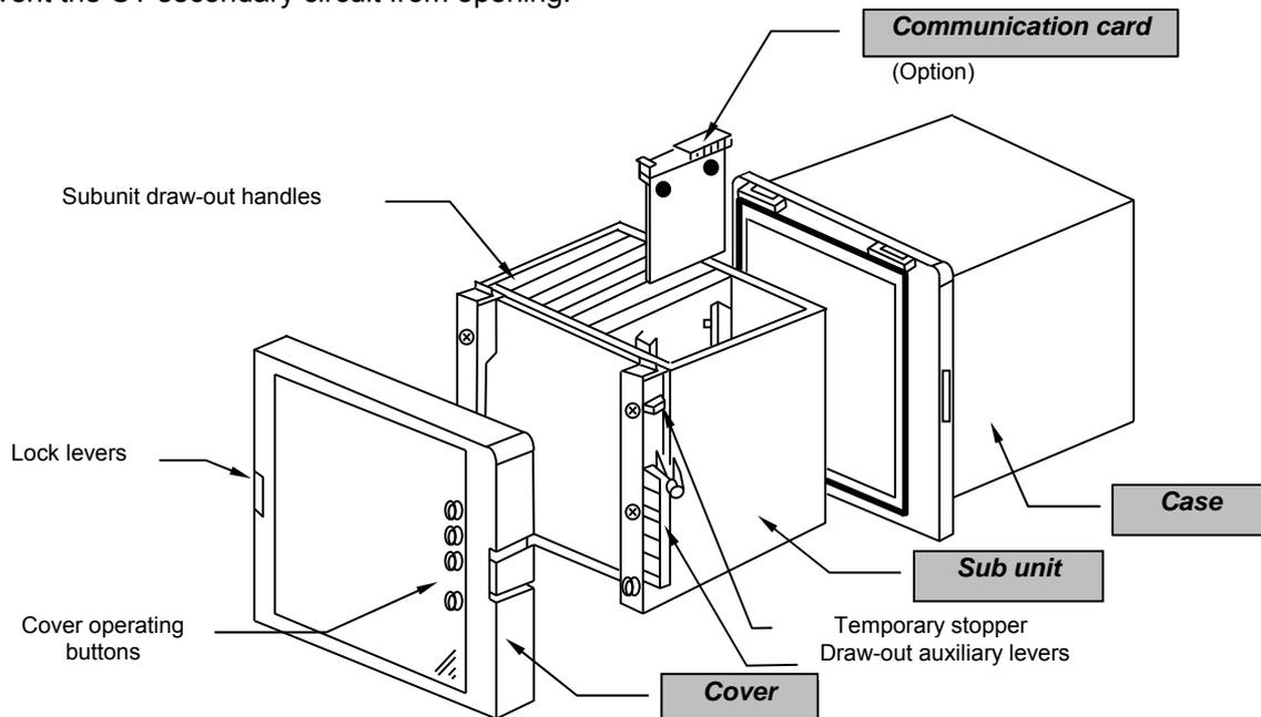
Figure 6-1 Outside view of type CGP2-A01D2 relay
