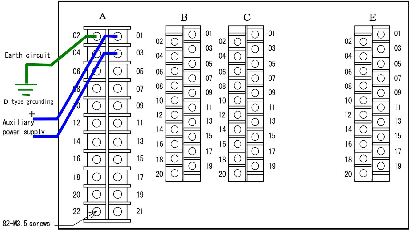
Figure 5-7 Rear view of type CGP2-A01D2 relay
