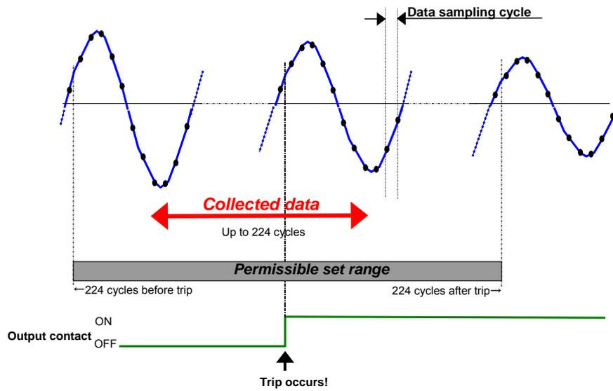
**Figure 4-15 Concept of recording fault waveform**
