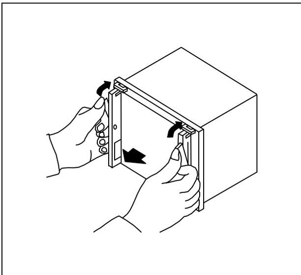
With the draw-out auxiliary levers touching the metallic parts, **exert your strength to turn round the levers** continuously, the sub unit will be drawn out a little from the case.
