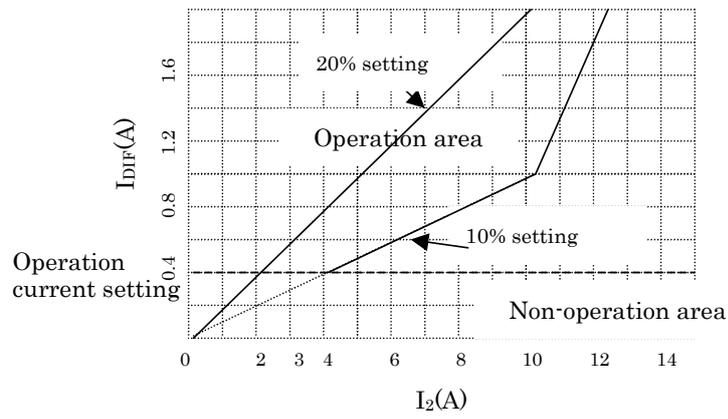
Figure 4-3 Biased differential characteristics between  $I_2$  and  $I_{DIF}$
