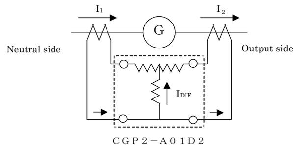
**Figure 4-1 Operating principle**
