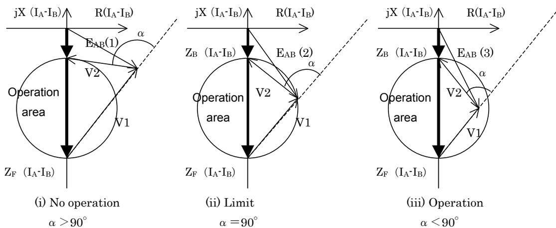
Figure 4-9 Operating principle (phase discriminating principle)
