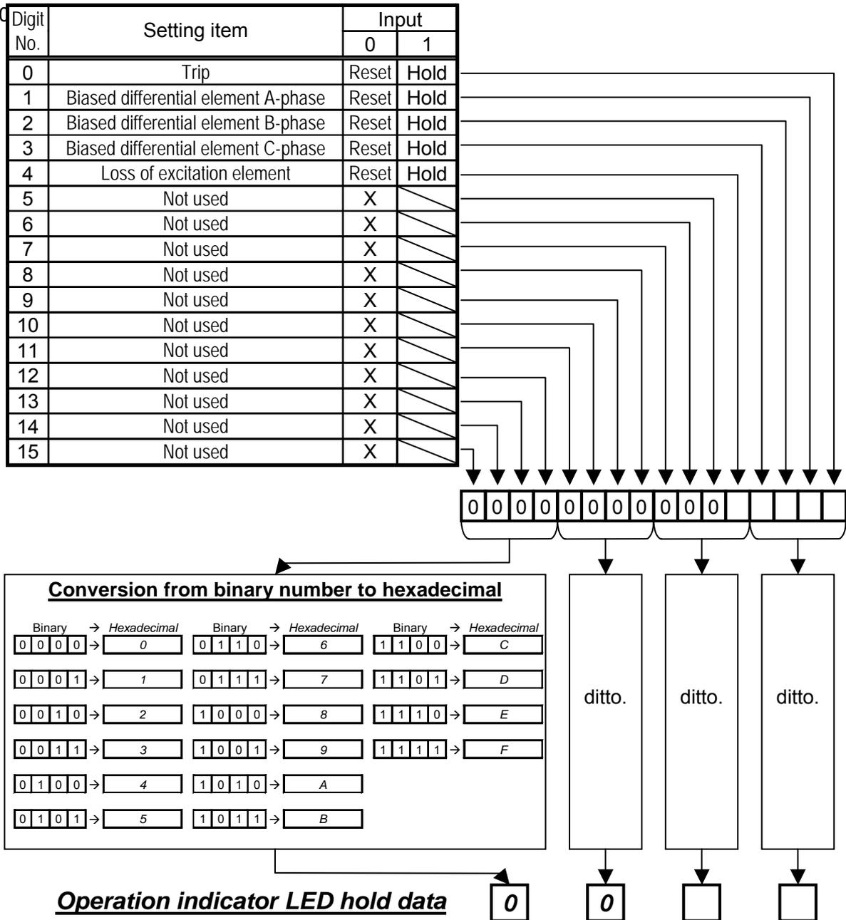
When the product is shipped from the factory, all LEDs are set to self-hold.
