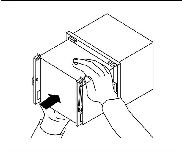
Hold the sub unit on the top and bottom to push the unit into the case approx. a half of the unit.
