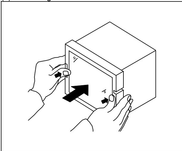
**Fit the cover straight** to the case. Hold the cover frame to **fully push the lock levers, located both side of the cover, to case side until it is clicked and locked.**
