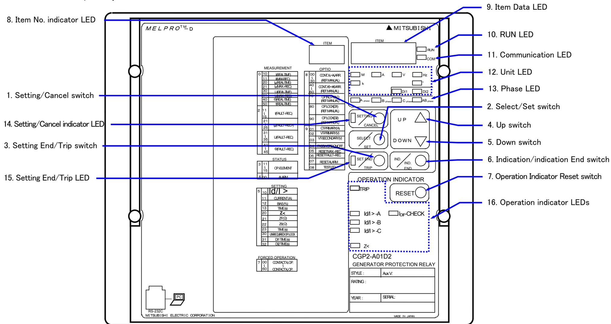
Figure 6.1 Front view of type CGP2-A01D2 relay
