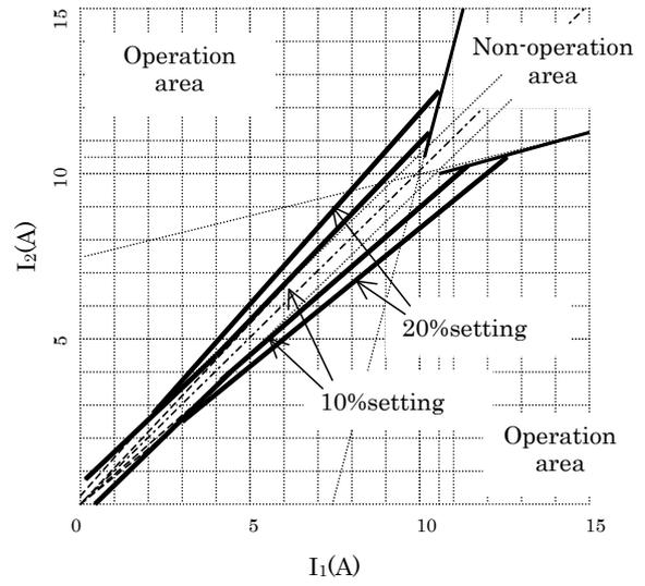
Figure 4-2 Biased differential characteristics between  $I_1$  and  $I_2$
