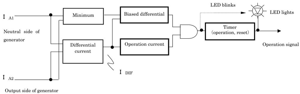
**Figure 4-4 Bias differential element function diagram (A-phase)**
