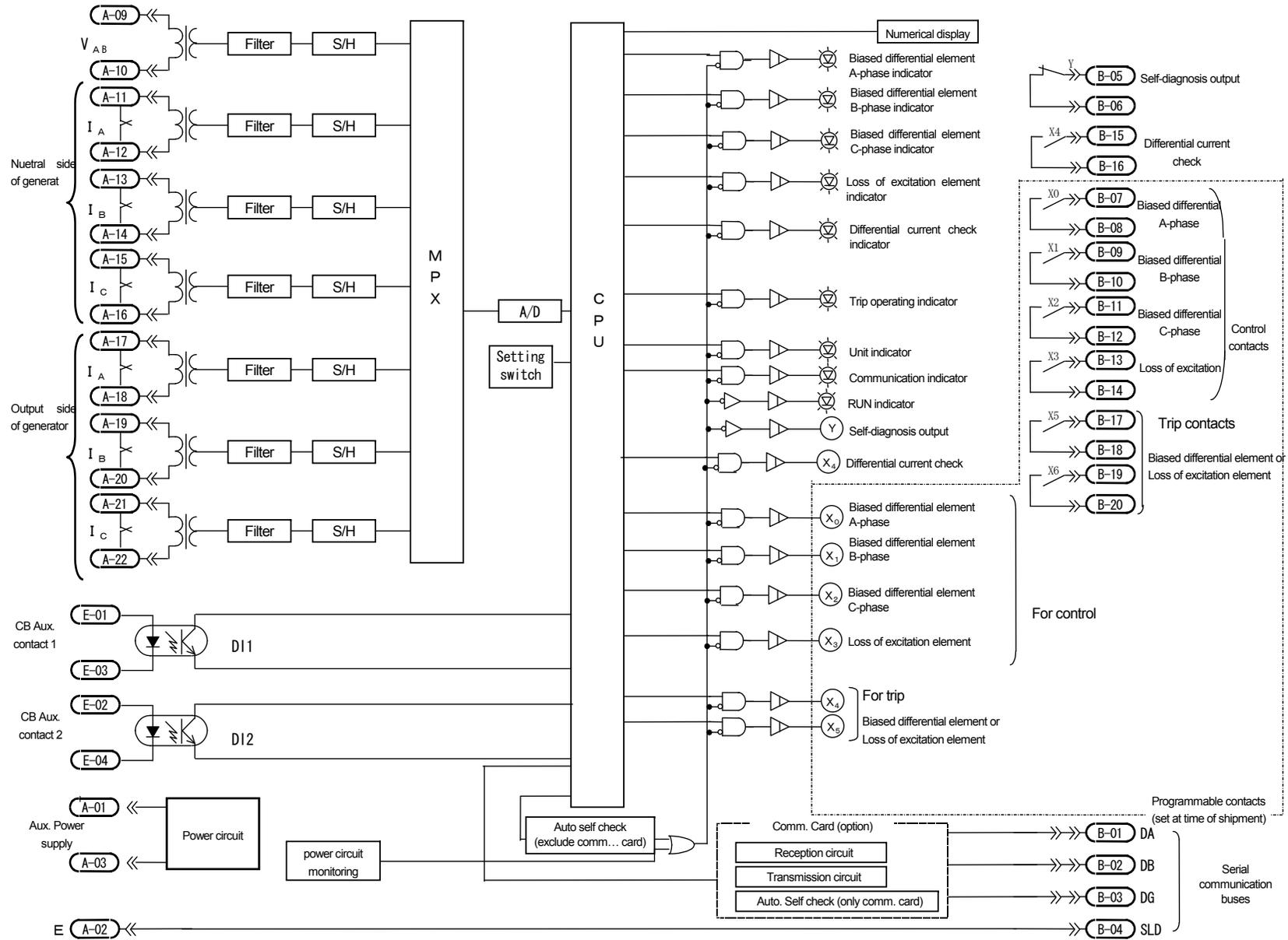
Figure 5-1 Internal block diagram of Type CGP2-A01D2 relay
