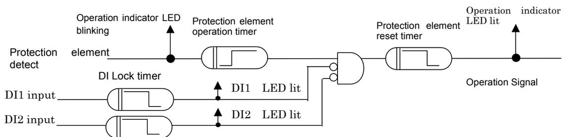
Figure 4-14 Example of Lock function by external control input
