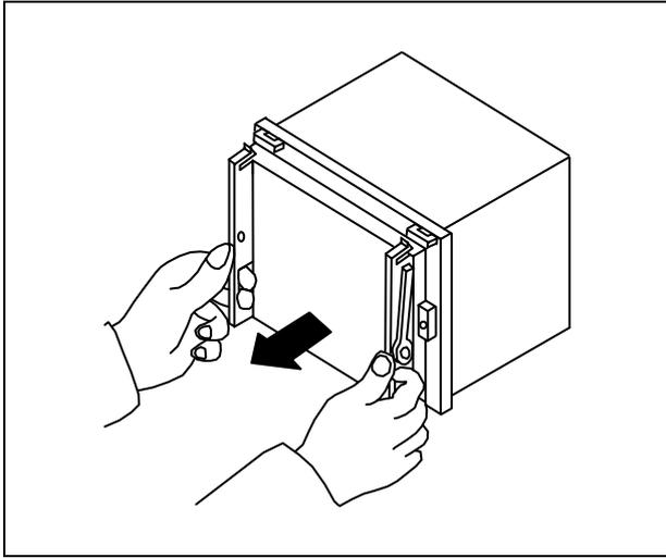
Grip the draw-out handles (located at both sides of the front of the sub unit), and **pull the sub unit towards you** until about a half portion of the sub unit is pulled out of the case.
