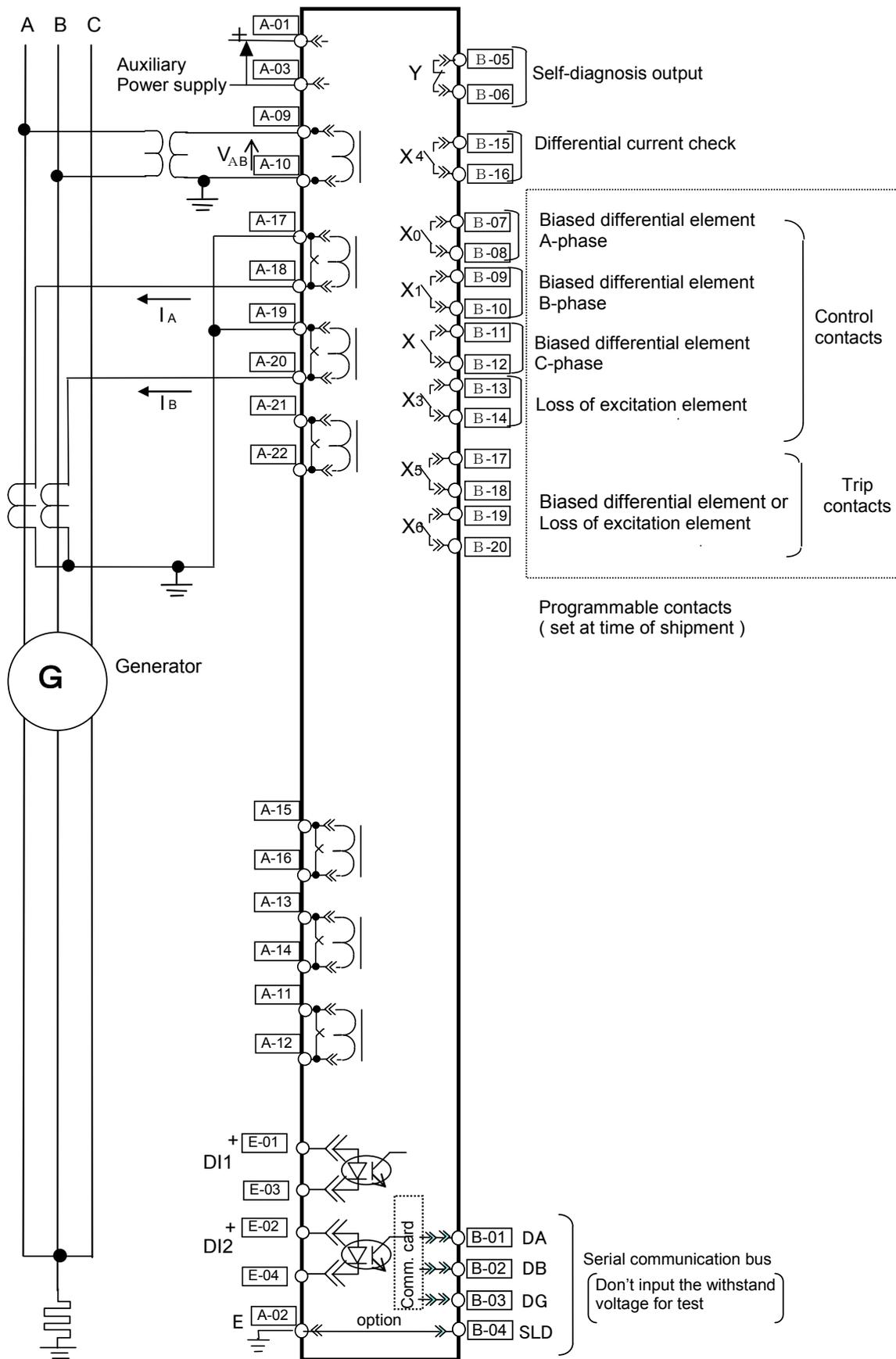
**Figure 5-5 External connection diagram for CGP2-A01D2 relay
