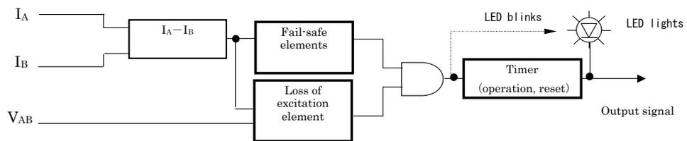
Figure 4-11 Loss of excitation element function diagram
