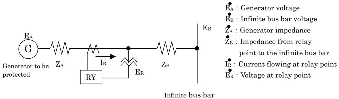
Figure 4-5 System diagram
