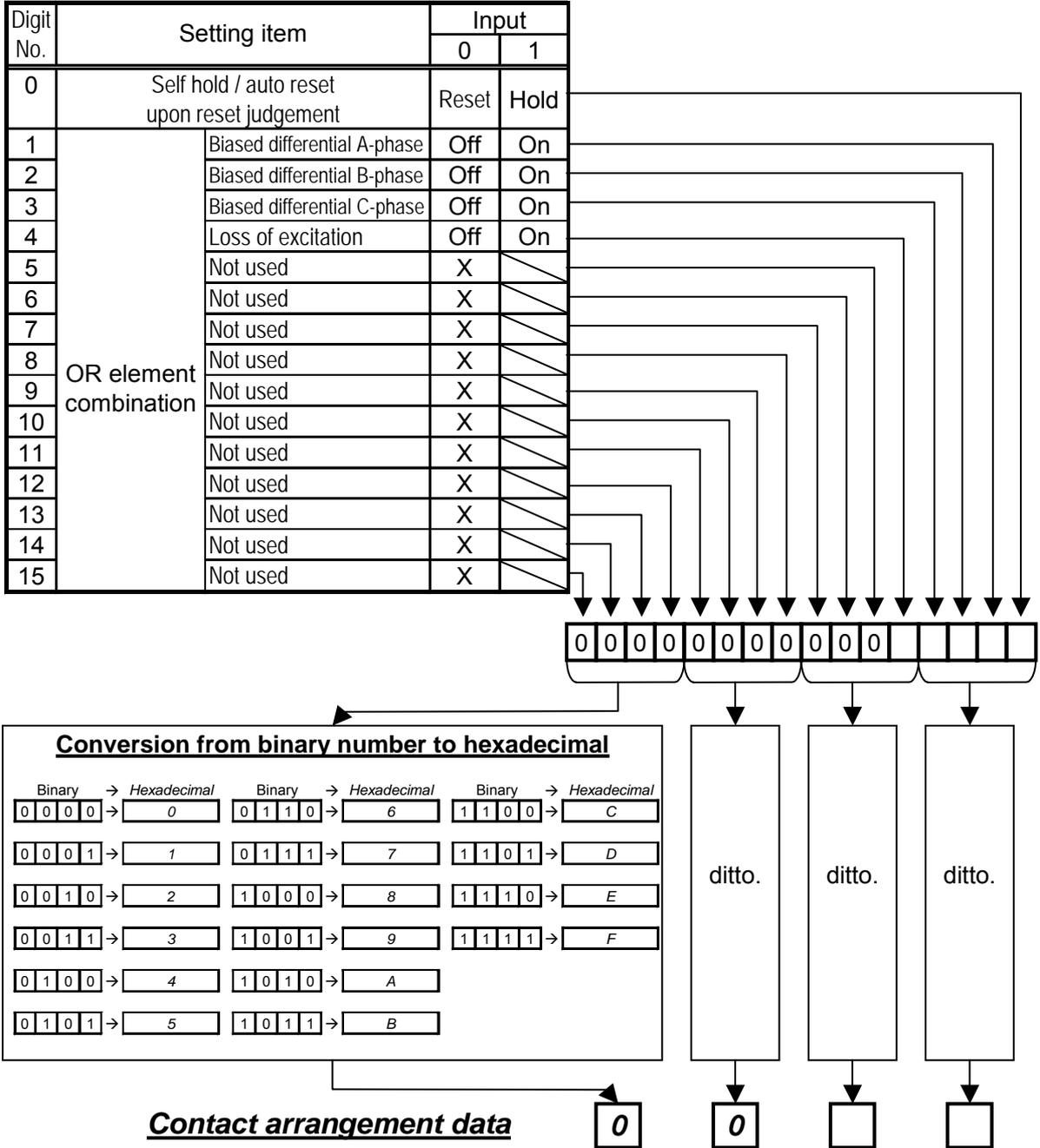
When the product is shipped from the factory, contact arrangement data are set as follows.
