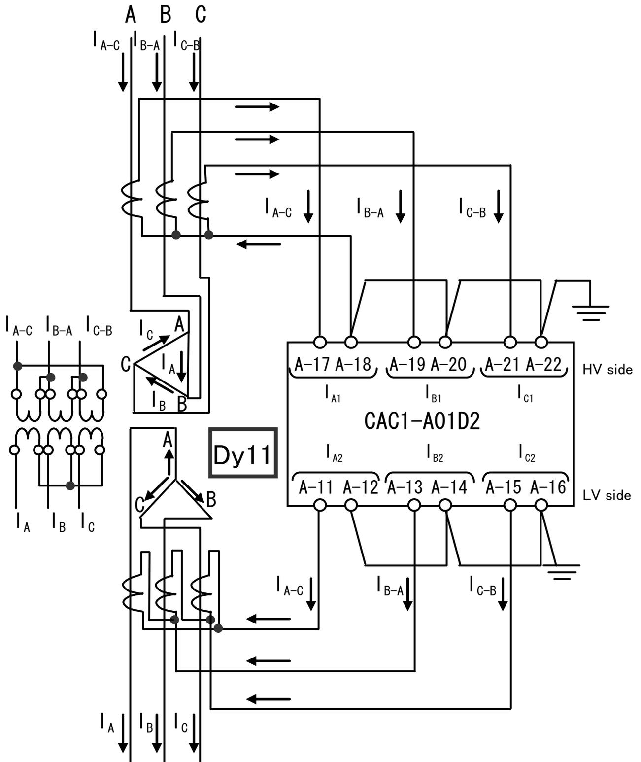
CT secondary circuit should be connected so as HV side current to be inflow to the Ry terminal of HV side and LV side current to be out flow from the Ry terminal of LVside with keeping same phase angle between bothside, when flow -through current is placed.
