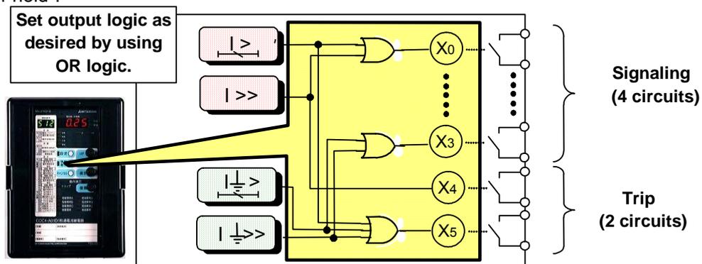
Figure 4.4 Schematic image of Programmable Outputs (example: COC4-A01D1)
