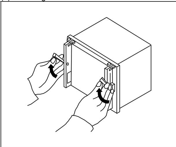
**Please from under to upper direction turn round the draw-out auxiliary levers** located on both sides of the front of the sub unit until the levers touch the metallic parts located on both sides of draw-out handles completely. **(Rotated angle is approx. 120°)**
