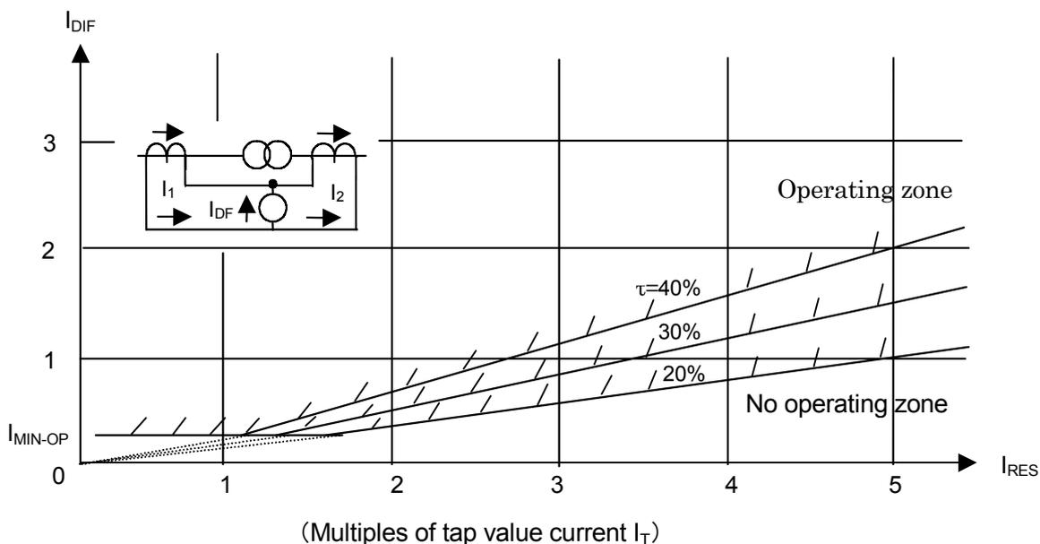
$$I_{DIF} : \text{Differential current } ( I_1 \cdot \frac{I_n}{I_{T1}} - I_2 \cdot \frac{I_n}{I_{T2}} )$$
