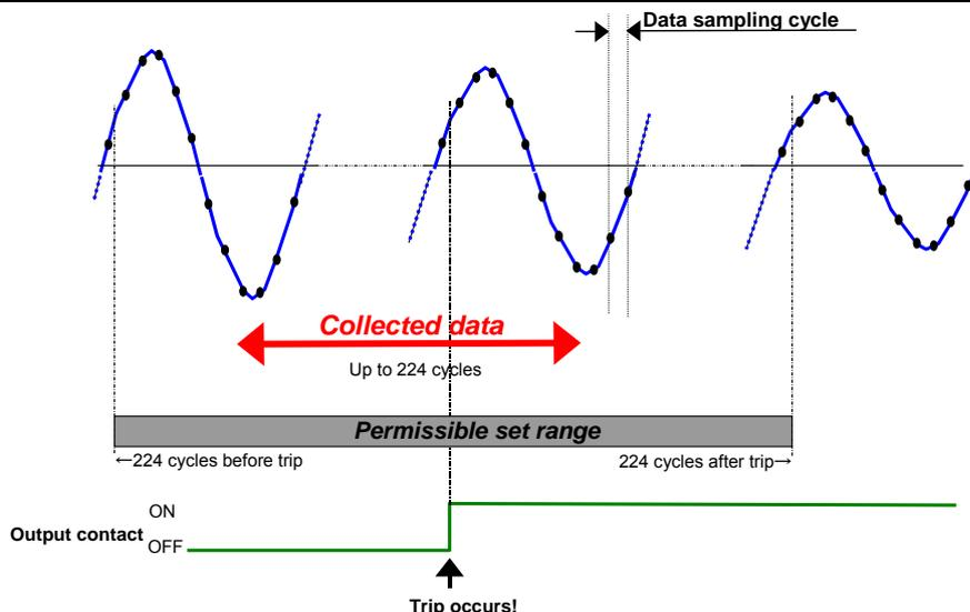
Figure 4.5 Recording concept of fault waveform
