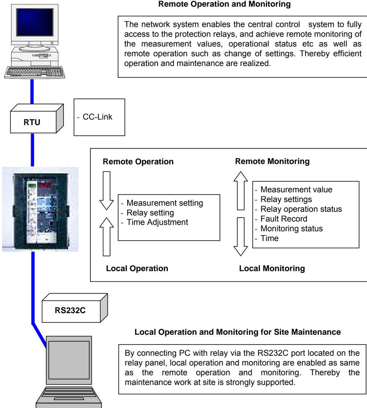
**Figure 4.6 Example of communication network system configuration**
