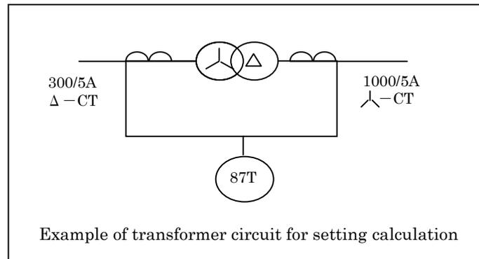
In order to set the relay correctly, please carry out the setting calculation as shown below and set the relay according to the calculation results.
