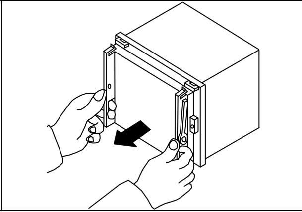
Grip the draw-out handles (located at both sides of the front of the sub unit), and **pull the sub unit towards you** until about a half portion of the sub unit is pulled out of the case.
