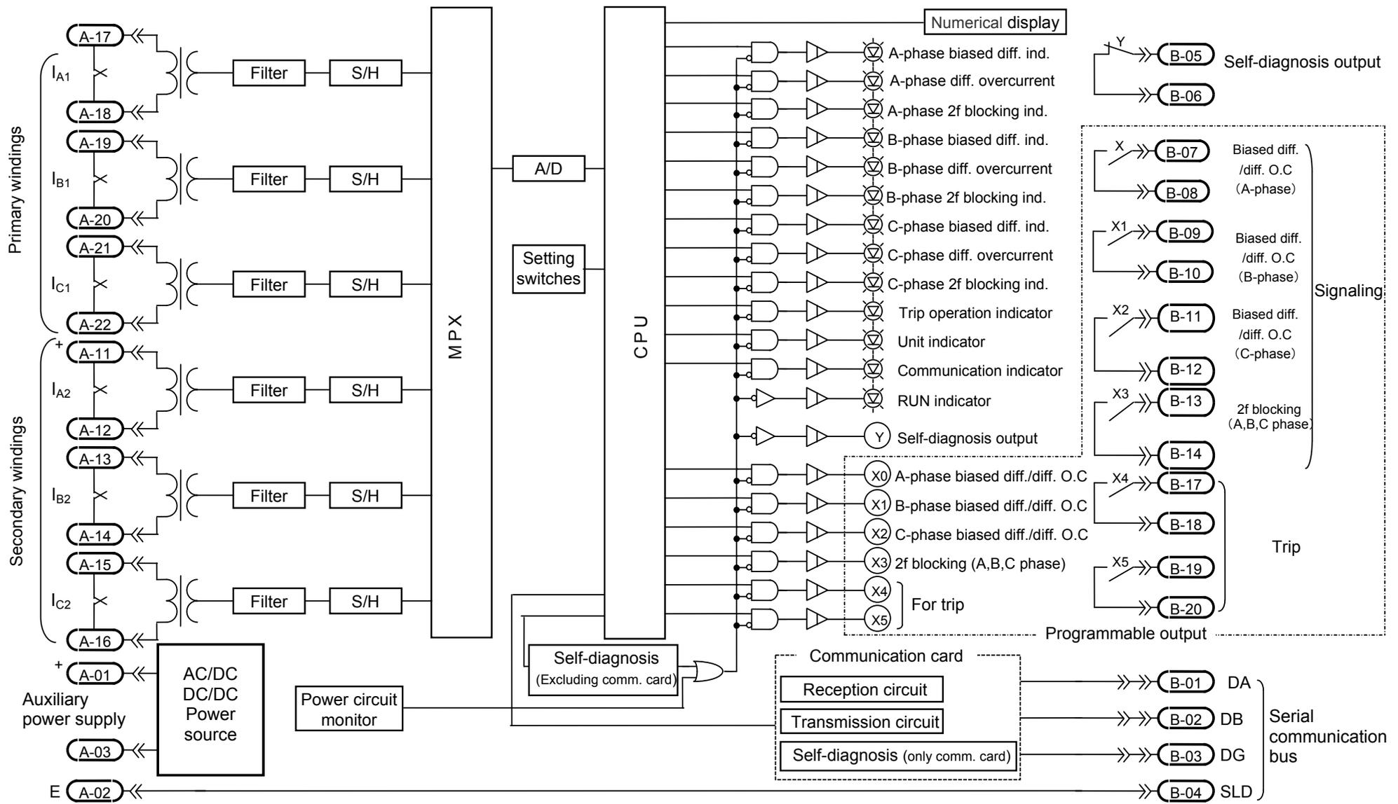
Figure 5.1 Internal block diagram of Type CAC1-A01D2 relay
