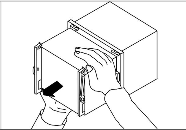
When about a half portion of the sub unit is pulled out of the case, just stop the drawing motion. Then, **hold the top and bottom of the sub unit to pull it out completely**, in order to prevent the unit from falling.
