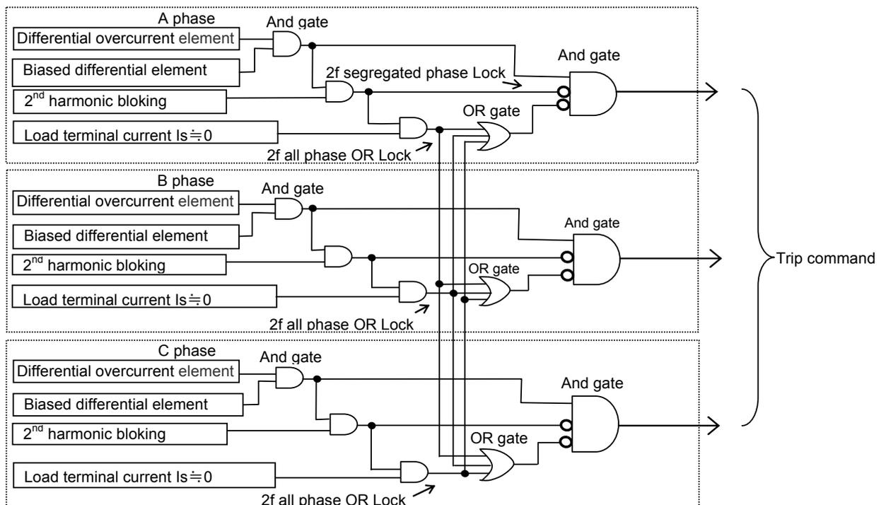
Figure4.3 Load terminal current  $I_s = 1/2 \times$  setting value of biased differential element
