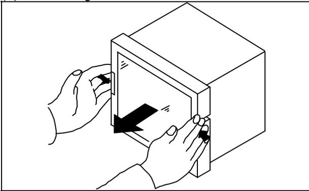
Hold the **lock levers**, which are located at both sides of the cover, on their front sections. Take off the cover **straight toward you** while pushing the levers **inwards**.
