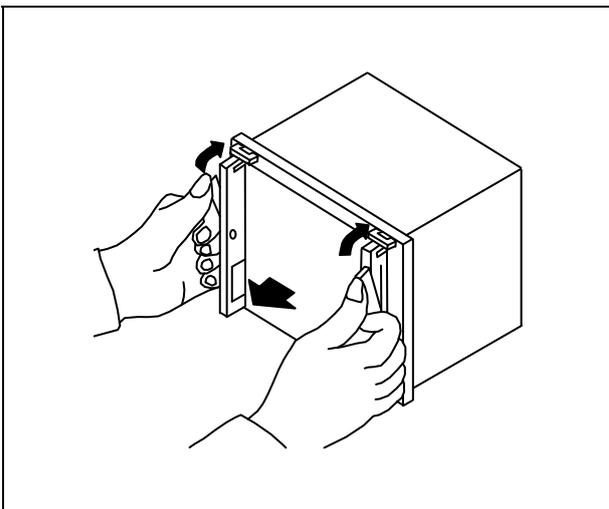
With the draw-out auxiliary levers touching the metallic parts, **exert your strength to turn round the levers** continuously, the sub unit will be drawn out a little from the case.
