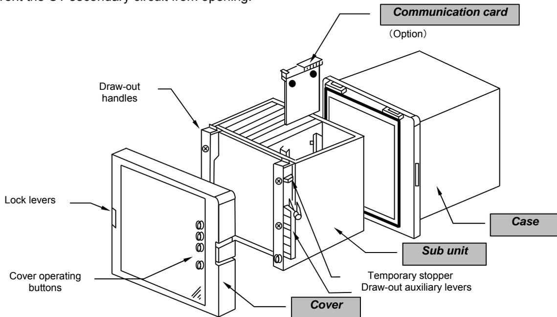
Figure 6.1 Outside view of type CAC1-A01D2 relay
