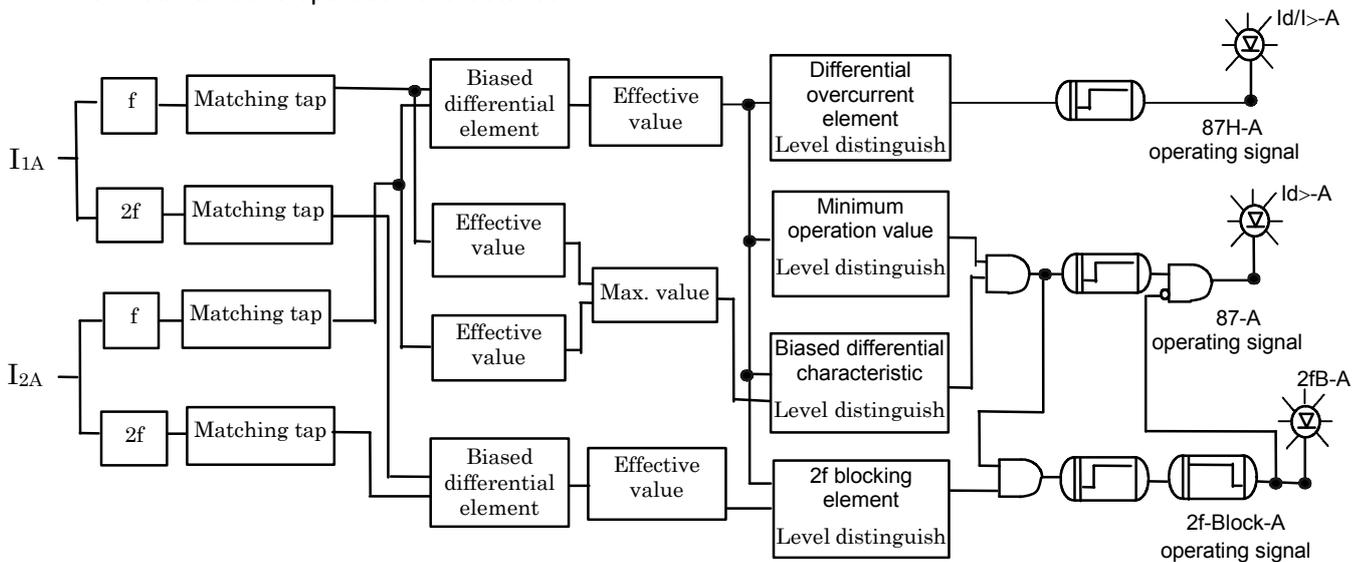
**Figure 4.1 Biased differential element • Differential overcurrent element Internal function diagram
