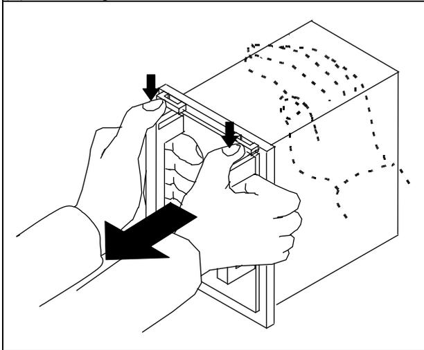
Grip the draw-out handles (located at both sides of the front of the sub unit). **Press the locking pieces installed in the upper portion of the draw-out handles with your thumbs to pull the sub unit towards you.**
