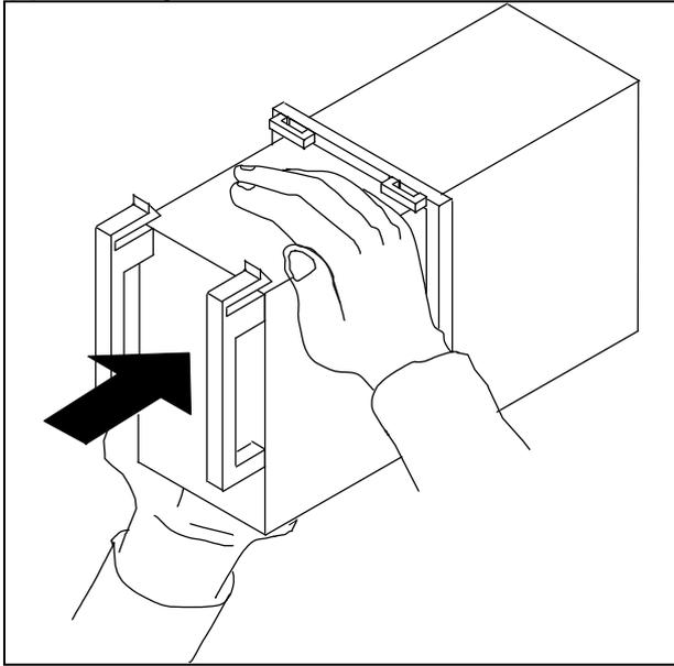
Hold the sub unit on the top and bottom to push the unit into the case approx. a half of the unit.
