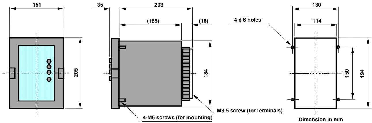
**Figure 7.1 Outside dimension /drilling drawing**
