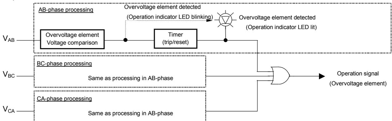
**Figure 4.2 Overvoltage element internal function diagram**
