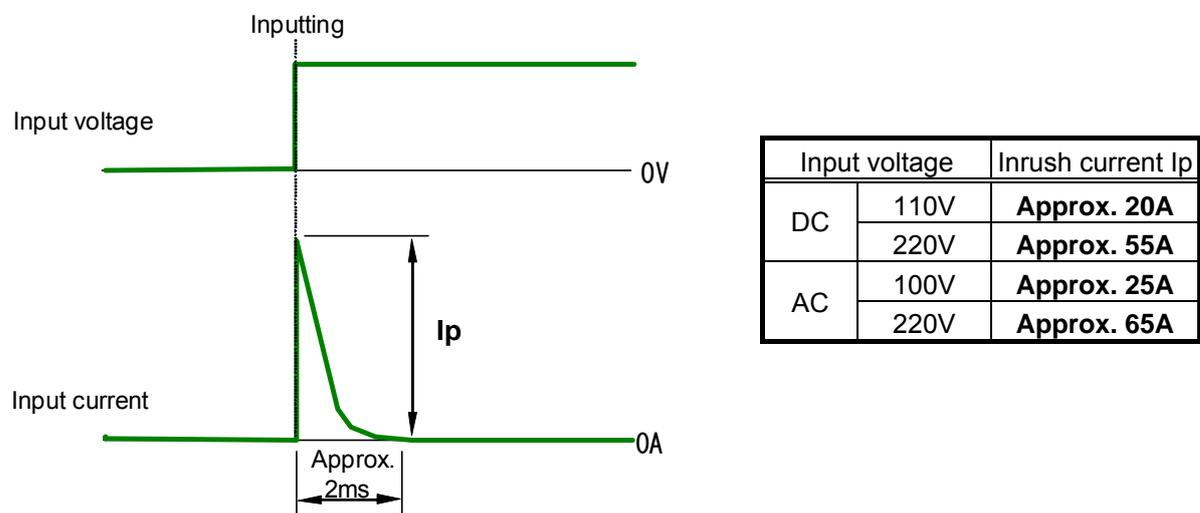
**Figure 5.3 Inrush current of auxiliary power supply**
