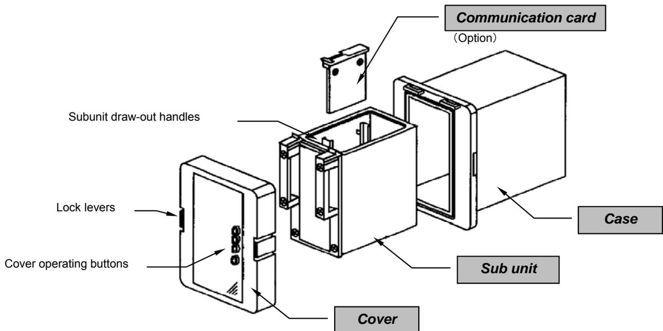
Figure 6.1 Outside view of type CBV2-A01D1 relay
