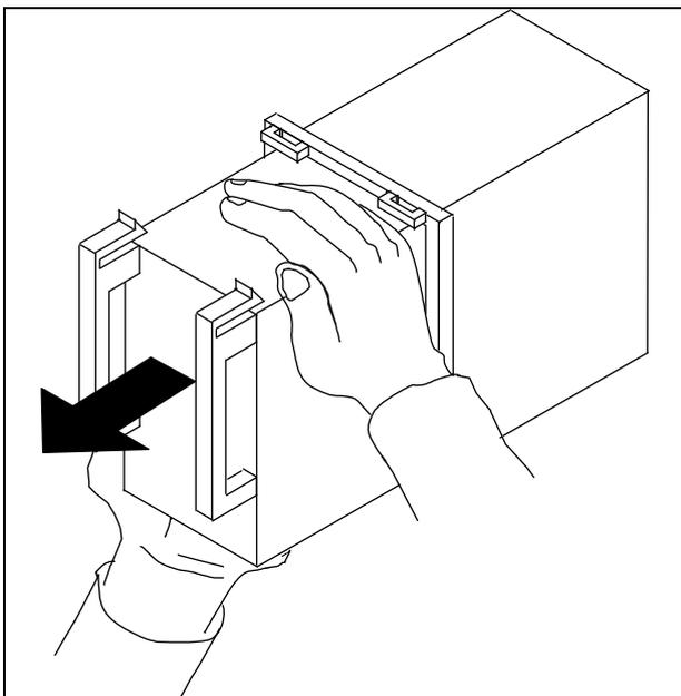
When about a half portion of the sub unit is pulled out of the case, just stop the drawing motion. Then, **hold the top and bottom of the sub unit to pull it out completely**, in order to prevent the unit from falling.
