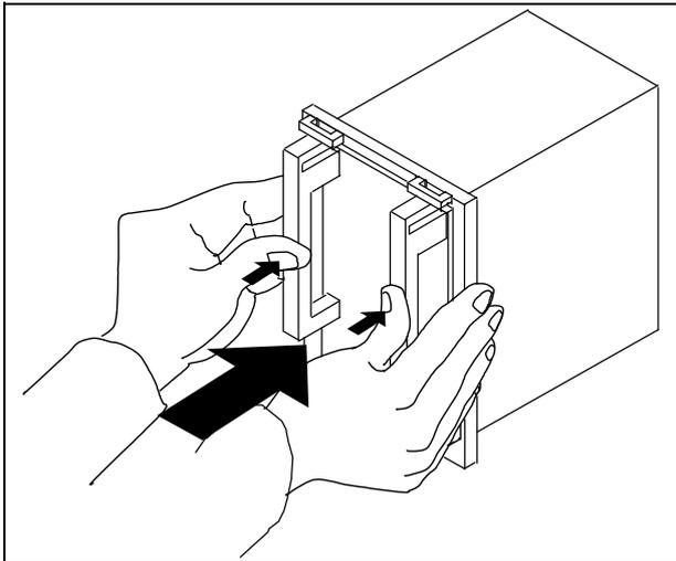
**Fully insert the sub unit into the case until you hear a click** while pressing the handles located on both sides of the front of the sub unit, and also the front face of subunit (ie, 4 corners of front face) is becoming flush with the vertical surface of the case.
