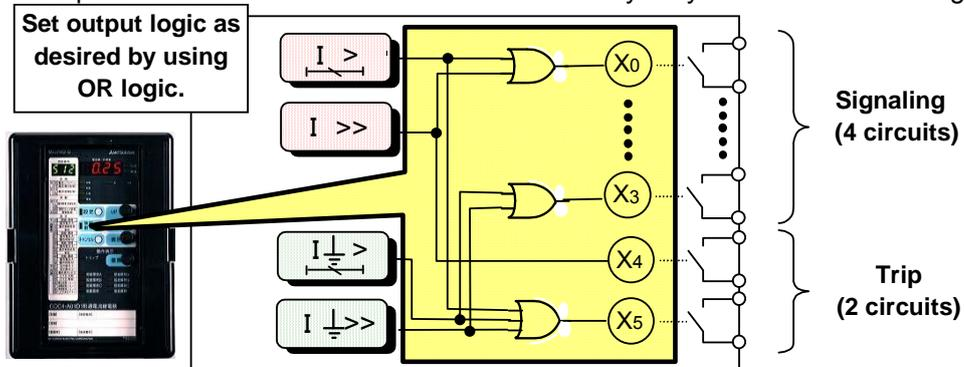
**Figure 4.3 Schematic image of Programmable Outputs (example: COC4-A01)**
