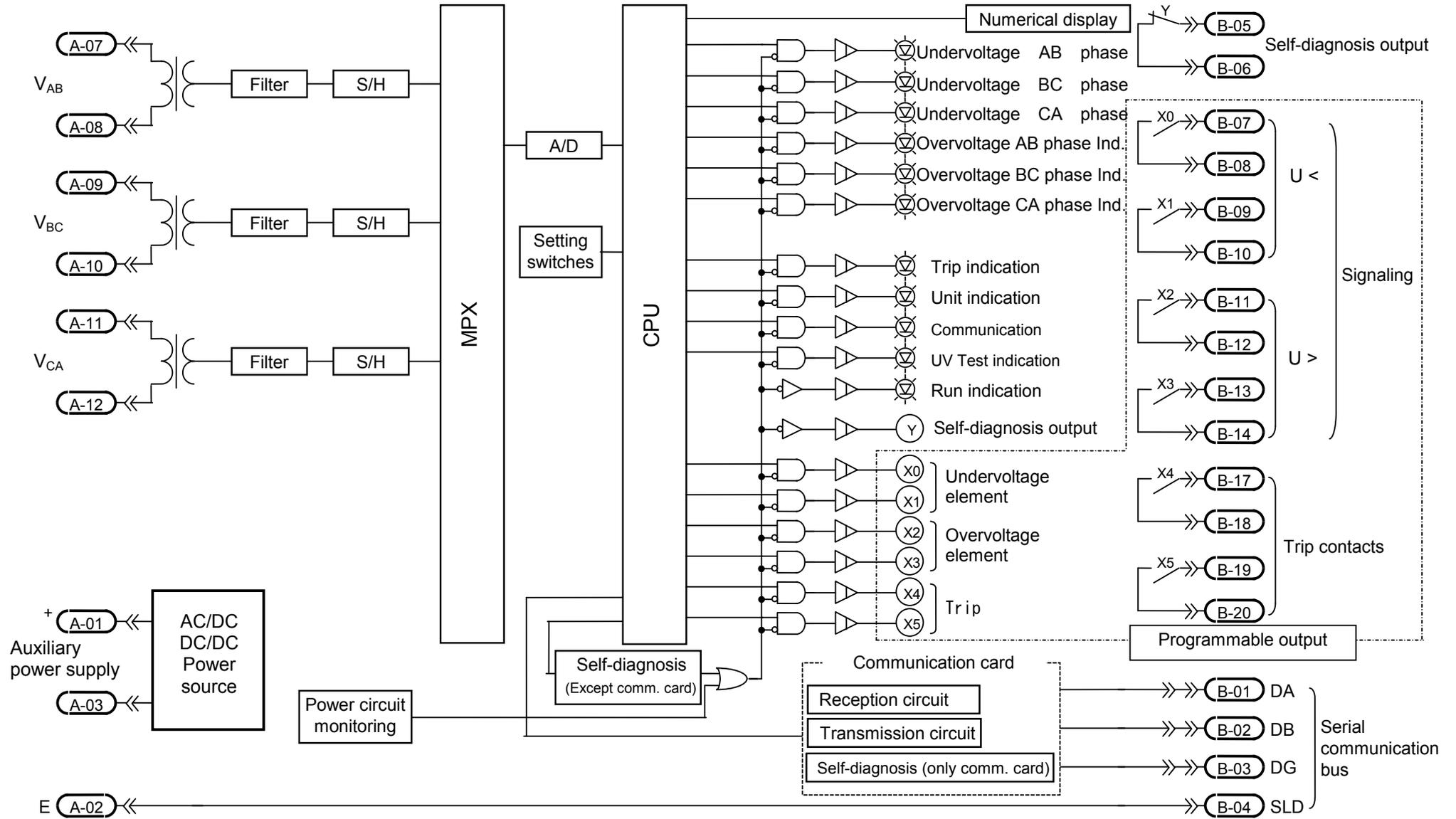
Figure 5.1 Internal block diagram of Type CBV2-A01D1 relay
