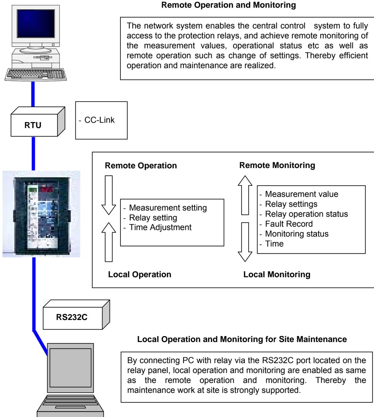
Figure 4.5 Example of communication network system configuration
