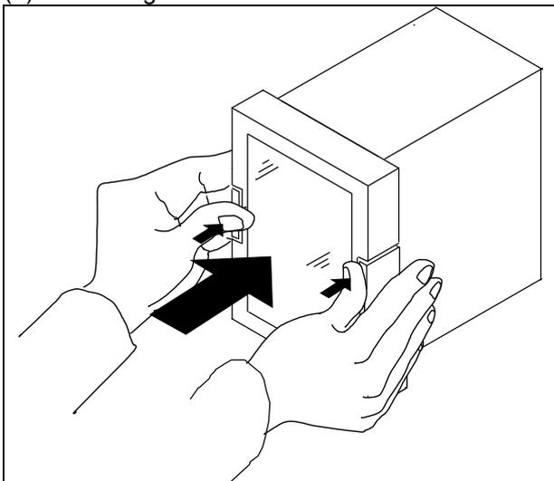
**Fit the cover straight** to the case. Hold the cover frame to **fully push the lock levers, located both side of the cover, to case side until it is clicked and locked.**
