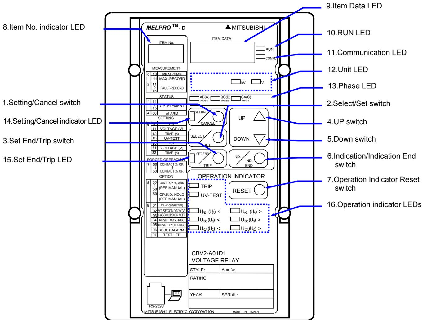
Figure 6.2 Front view of type CBV2-A01D1 relay
