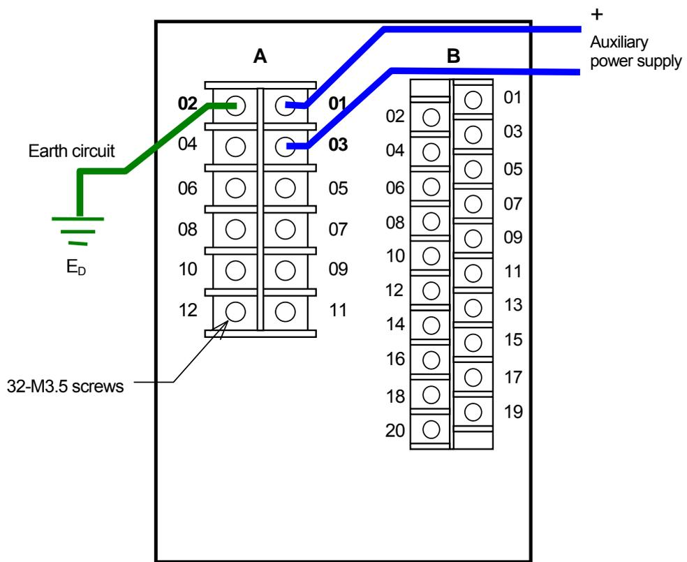
Figure 5.6 Rear view of type CBV2-A01D1 relay
