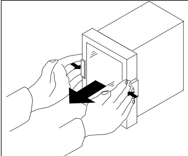
Hold the **lock levers**, which are located at both sides of the cover, on their front sections. Take off the cover **straight toward you** while pushing the levers **inwards**.
