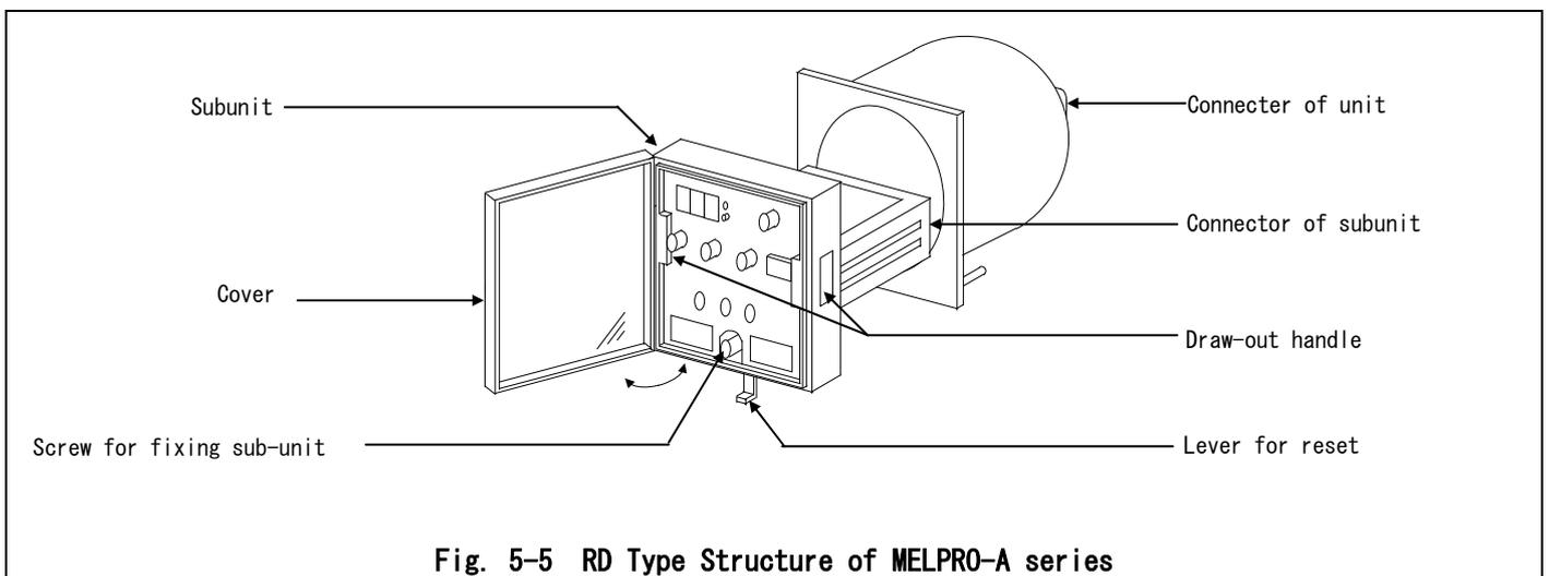
Fig. 5-5 RD Type Structure of MELPRO-A series
