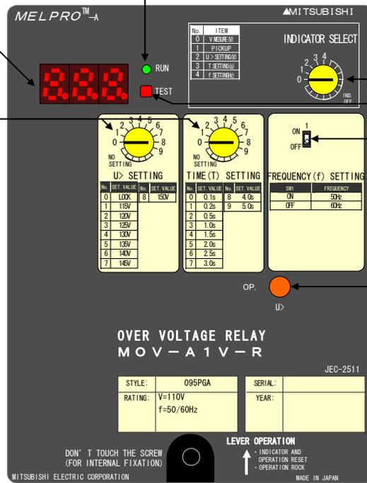
Fig. 5-1 MOV-A1 series construction (panel)
