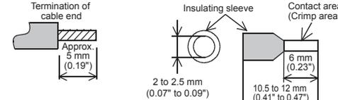
When using a ferrule with insulation sleeve, choose a wire with proper cable sheath referring to the above outside dimensions, otherwise the wire cannot be inserted easily.
