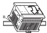
3) Lock the DIN rail mounting hooks (below fig. C) while pressing the PLC against the DIN rail.
