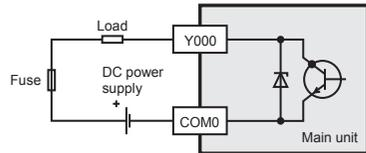
**2. External wiring of source output type**
