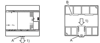
2) Fit the upper edge of the DIN rail mounting groove (right fig. B) onto the DIN rail.
