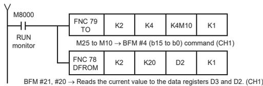
The following programs are the examples of error processing. Error status in the FX3U-2HC can be checked by reading the contents of b0 to b15 of BFM #29 to auxiliary relays of the PLC. These error flags are resettable BFM #4, #44 b8.
