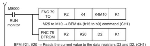
The following programs are the examples of error processing. Error status in the FX3U-2HC can be checked by reading the contents of b0 to b15 of BFM #29 to auxiliary relays of the PLC. These error flags are resettable BFM #4, #44 b8.
