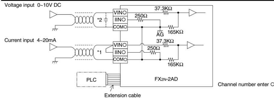
\*1 The FX<sub>2N</sub>-2AD cannot have 1 channel as an analog voltage input and one channel as current input because both channels use the same offset and gain values. For current input please short circuit VIN and IIN as shown in the diagram.
