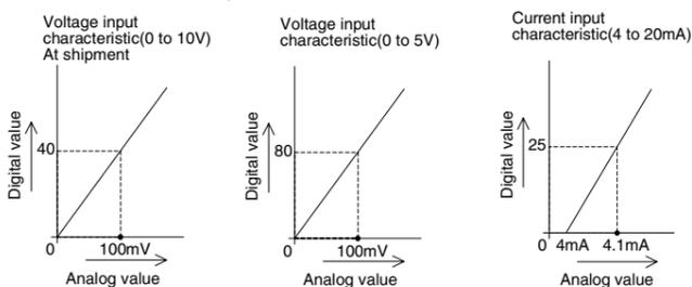
For instance, when a digital range of 0 to 4000 is used with the analog range of 0 to 10V, a digital value of 40 is equal to an analog input of 100mV. ( $40 \times 10V/4000$  digital points)
