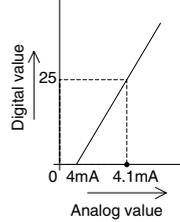
For instance, when a digital range of 0 to 4000 is used with the analog range of 0 to 10V, a digital value of 40 is equal to an analog input of 100mV. ( $40 \times 10V/4000$  digital points)
