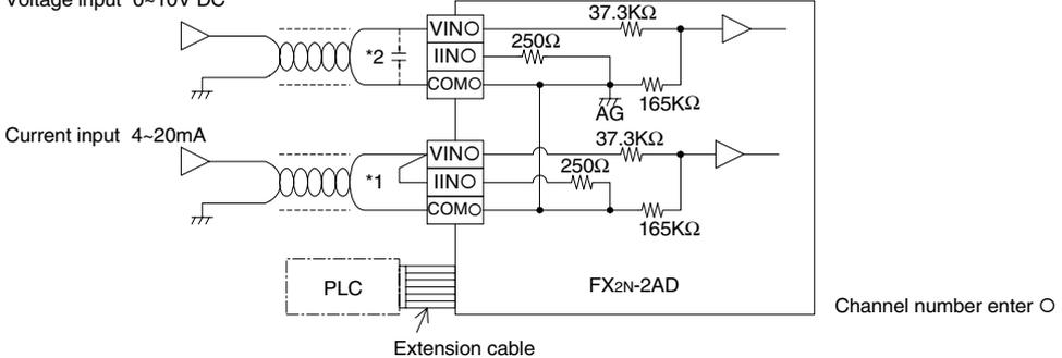
\*1 The FX2N-2AD cannot have 1 channel as an analog voltage input and one channel as current input because both channels use the same offset and gain values. For current input please short circuit VIN and IIN as shown in the diagram.
