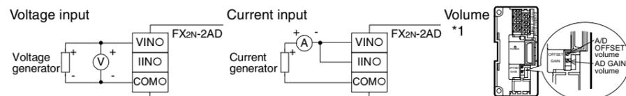
\*1 The digital value increases if the volume is turned clockwise. (FX2N-4DA and FX2N-2DA can be used instead of the voltage and current generator)
