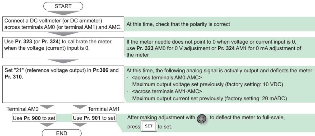
In **Pr. 306** and **Pr. 310**, set the types of the signals to be output. (Refer to [page 26](#).)
