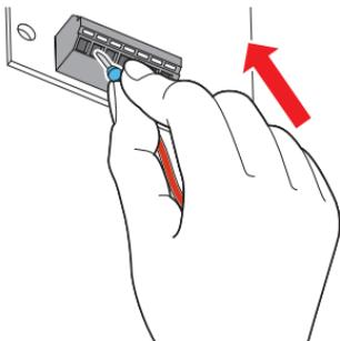
When using a single wire or stranded wires without a blade terminal, push the open/close button all the way down with a flathead screwdriver, and insert the wire.
