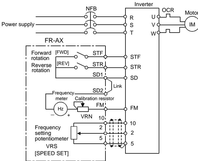
Fig. 4 Connection Diagram and Wiring Example
