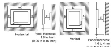
According to the dimensions in the following table, leave clearances between the GOT and the other devices. The values enclosed in square brackets apply to the case where no other equipment generating radiated noise (such as a contactor) or heat is installed near the GOT. However, keep the ambient temperature of the GOT to 55°C or lower.
