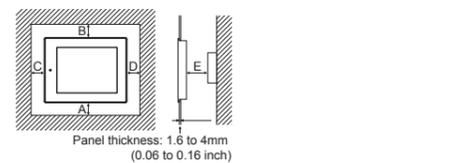
According to the dimensions in the following table, leave clearances between the GOT and the other devices. The values enclosed in square brackets apply to the case where no other equipment generating radiated noise (such as a contactor) or heat is installed near the GOT.
