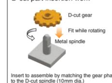
Insert to assemble by matching the gear phase to the D-cut spindle (10mm dia.)
