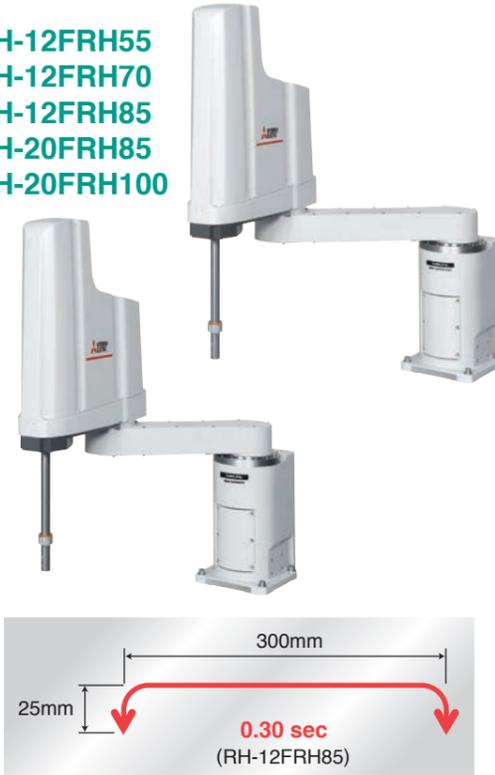
A horizontal, multiple-joint type robot with highly rigid arms and cutting-edge servo controls to provide extremely fast and precise heavy-duty operation. Enhancements to the wrist axis also mean that the robot has ample scope for handling multi-function grippers and offset grippers. Ideal for assembly and palletizing work.
