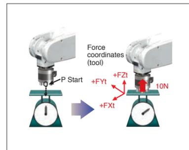
Keeps the force constant so that the workpiece can be handled without causing damage
