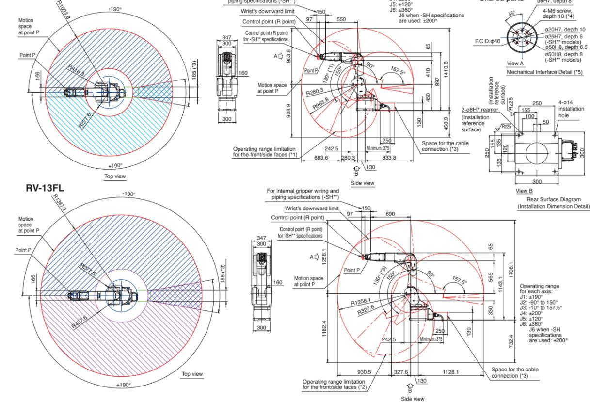
\*1: Operating range for the front and side parts: When the J1-axis angle is inside the range of J1±120° or J1±130°, the operating range of the J2-axis is limited to -90°±J2 ±130°.
