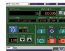
The robot operations screen provides the same functions as the robot controller panel, and may be used to activate such automated operations as servo on/off, startup, shut-down, reset, and program selection.
