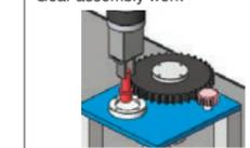
Assembly by meshing a flat gear and pinion gear
