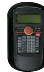
Used for creating, editing and managing programs, to teach operating positions and for jogging. Fitted with a 3-position enabling switch to ensure safe use. When multiple robots are used, the connections can be switched to a single teaching box. The connections can be switched when the power is shut off.
