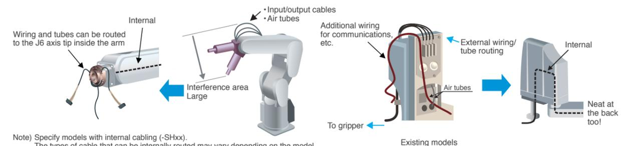
Note) Specify models with internal cabling (-SHxx). The types of cable that can be internally routed may vary depending on the model.
