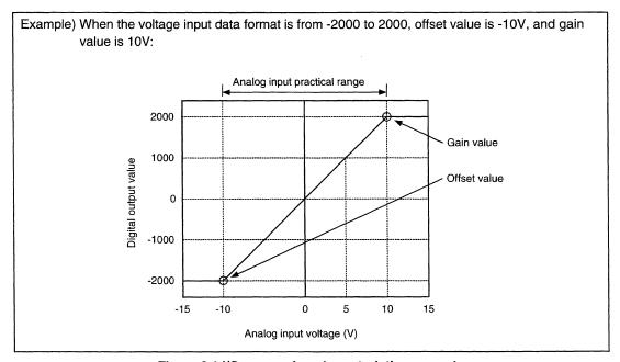
Figure 3.1 I/O conversion characteristics example
