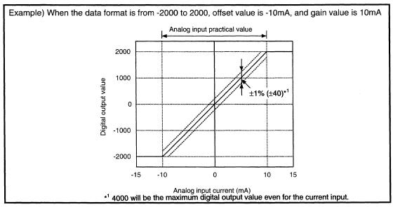
Figure 3.5 Total precision of the current input characteristic
