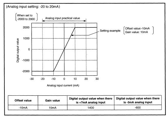
Figure 3.3 Current input characteristics
