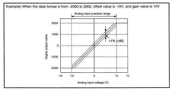
Figure 3.4 Total precision of the voltage input characteristic
