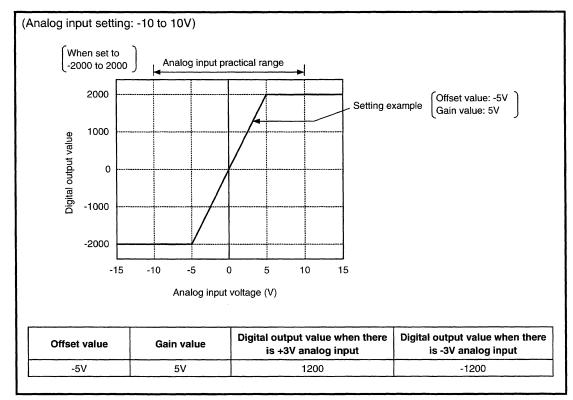
Figure 3.2 Voltage input characteristics
