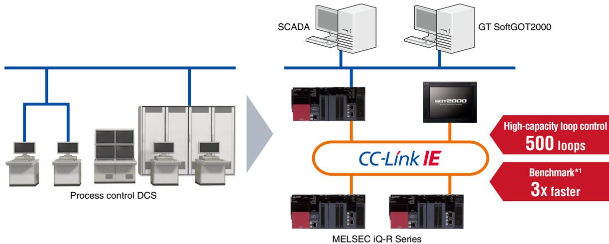
\*1: Based on a typical application example, the benchmark test measures the scan time taking into consideration the network refresh time and processing time of basic instructions and loop control, etc., and as compared to MELSEC-Q Series Process CPU (QnPHCPU).
