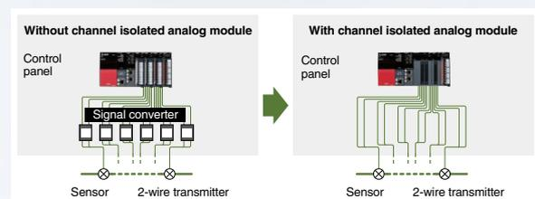
Electric disturbances such as current and noise can be isolated.
