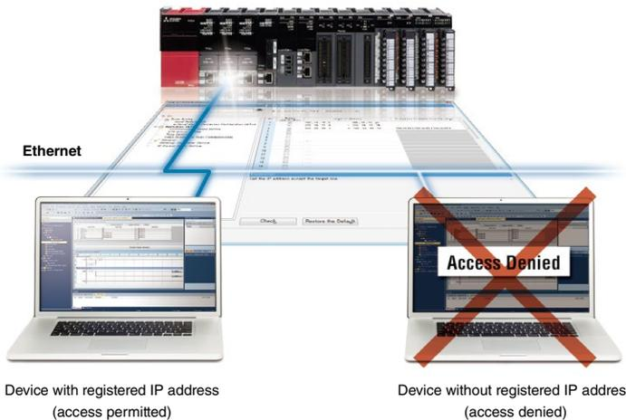
The IP filter can be used to register the IP addresses of devices permitted to access the CPU module. As a result, access from non-registered devices can be blocked, thereby lowering the risk of program hacking and unauthorized access by a third party. Another feature is a remote password function for password-based security. Passwords of up to 32 characters can be set to prevent unauthorized access to the CPU module via networks such as Ethernet.
