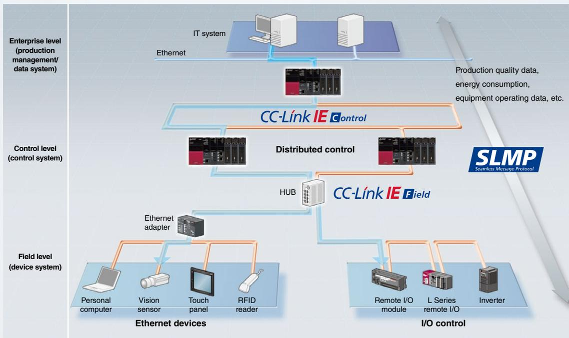
\*1: SLMP (Seamless Message Protocol): Is a client/server protocol that enables communications between Ethernet-ready and CC-Link IE compatible devices.
