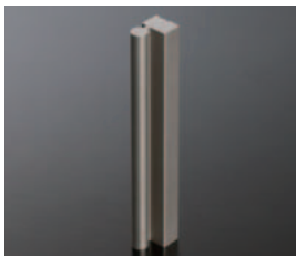
Wire electrode : \phi 0.2(.008) /BS Workpiece : Steel(SKD11), t60mm(2.4") Surface roughness : Rz3.5 \mu m/Ra0.45 \mu m/18 \mu "Ra
