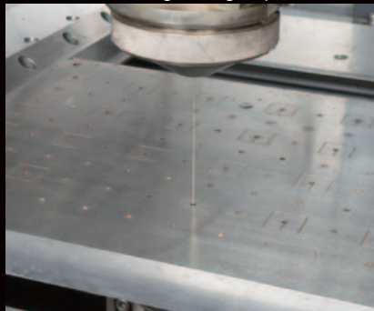
Stable automatic threading is realized during pitch machining
